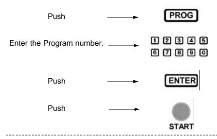
After the <u>ENTER</u> key has been pushed, the data in step 1 will be displayed along with the program number.
